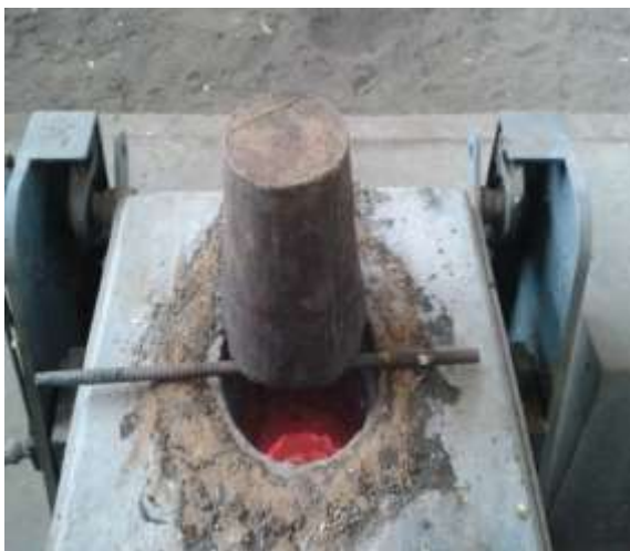
melting of low carbon steel
