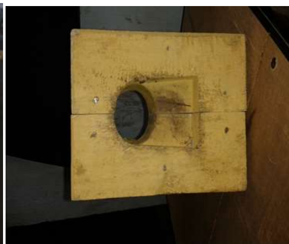
making corebox with coreprint
