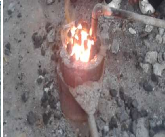
preheat of ladle
